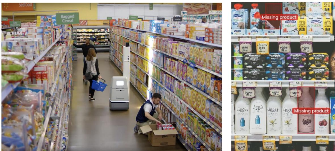
Figure 3: An AI autonomous robot powered by edge computing scanning inventory levels and planogram compliance while customers shop and Team Members work.
